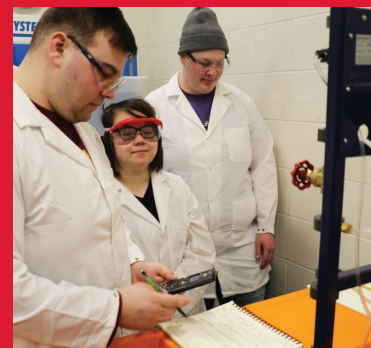
Students in ChE 160 collect pressure drop data with a flow meter demonstration unit purchased with a gift from Gary and Mickie Griswold .
