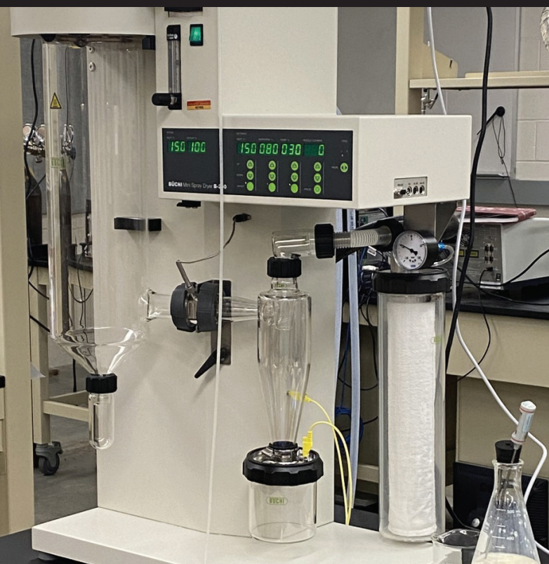
This spray dryer, purchased with alumni funds to support teaching and research experiments, aids in forming powders and particles.
