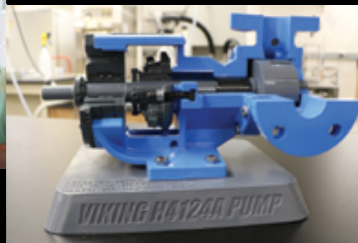
A 3D printed cutaway of a Viking internal gear pump used in industry has become part of a CBE lab as a teaching aid. CBE professor of practice John Kaiser and Viking Pump worked together to make the donation happen.
